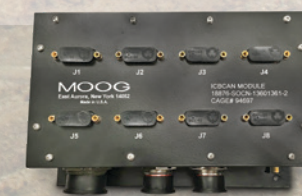
CONTROLLER AREA NETWORK SPLITTER
